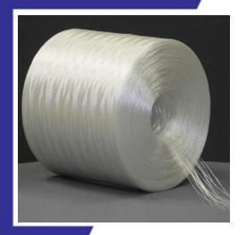
**FGOC ECPlus Spray-up Roving 221** is produced with **ECPlus** boron free-glass filament strands, gathered into a single bundle, and wound on a cylindrical package with even tension and without twist. The glass filaments are coated with a proprietary silane sizing system and provide
