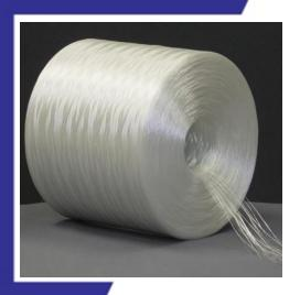
**FGOC ECPlus Chop Roving 241** is produced with **ECPlus** boron free-glass filament strands, gathered into a single bundle, and wound on a cylindrical package with even tension and without twist. The glass filaments are coated with a proprietary silane sizing system and provide
